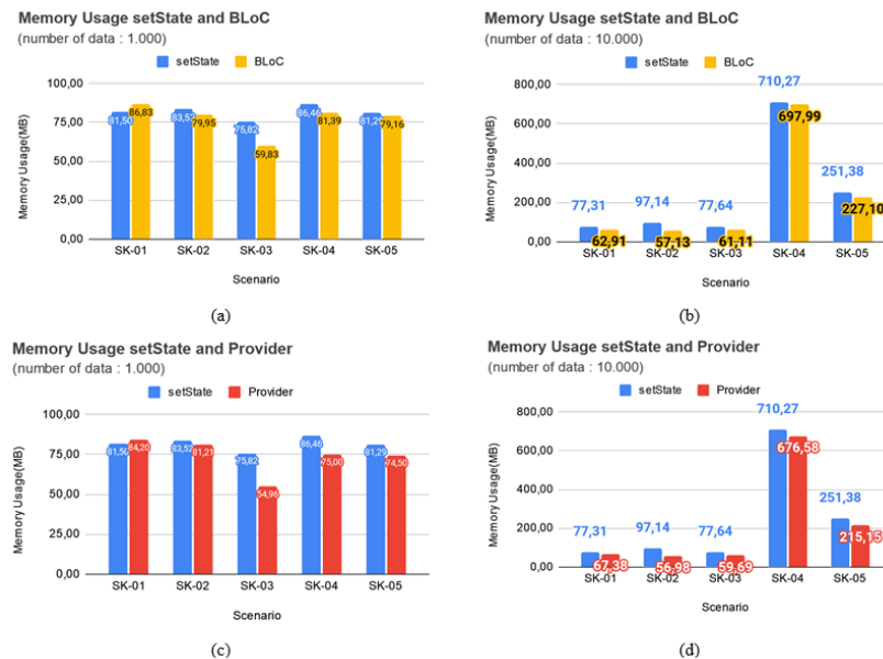
Fig 5. Memory usage comparison of (a)(b)setState and BLoC, (c)(d) setState and Provider
